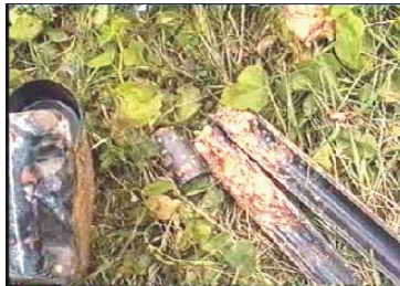
SPT samples as obtained from Wash bores
