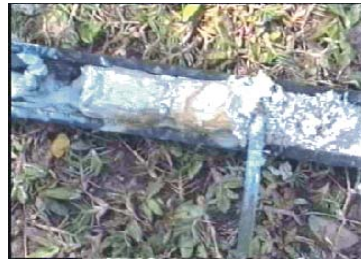
SPT samples as obtained from Wash bores
