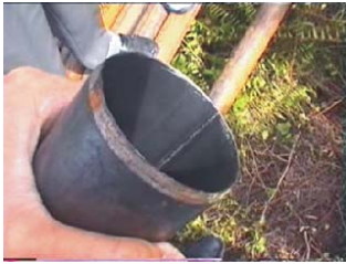
Commonly used Undisturbed sampling tube with obstruction on the inside □
