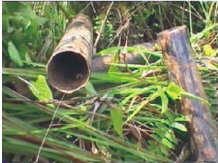
Badly damaged Undisturbed sampling tube
