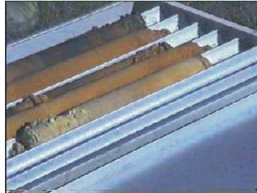
SPT Samples as obtained using proper boring methods
