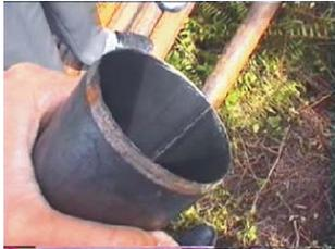
Commonly used Undisturbed sampling tube with obstruction on the inside ☐
