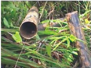
Badly damaged Undisturbed sampling tube
